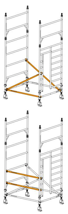
Fit an AGR on both sides of the tower. The top hooks of the AGR must be fitted to the top rungs of the 2 rung frame as shown.
