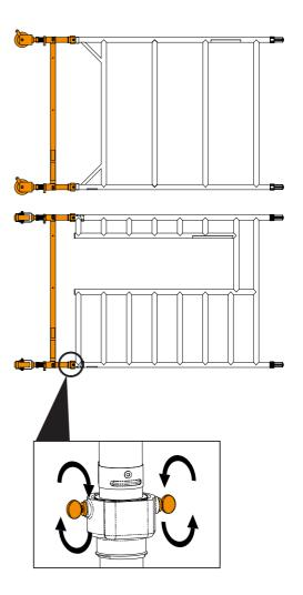
Fit one 2 rung span frame to the top of the walk-through assembly. Ensure interlock clips are connecting the frames together.
