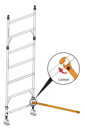
Position walk-through frame assembly as shown and fit the other end of the horizontal brace onto the vertical, just above the bottom rung.
