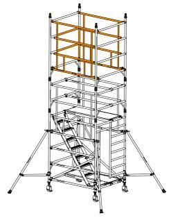
Standing on the fully guard-railed platform, fit the next staircase above and aligned with the first staircase with the landing claws fitted to the top cross member of the walk-through frame as shown.
