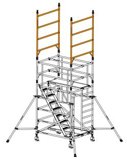
11 Fit an AGR on both sides of the tower. The top hooks of the AGR must be fitted to the top rungs of the 4 rung frame as shown.
