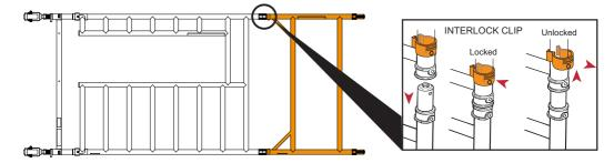
Fit one horizontal brace (red) onto the vertical of the span frame assembly, just above the bottom rung of the master rung, with the claw facing outwards. The frame will now be self-supporting.
