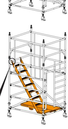
Fit a fixed deck to the top rung of the walk-through frame, directly above the lower fixed deck. Ensure the deck wind latches are engaged.
