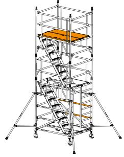
Continue the procedure until the required working height is reached, adding additional end frames, AGRs and staircases as shown on previous steps.
